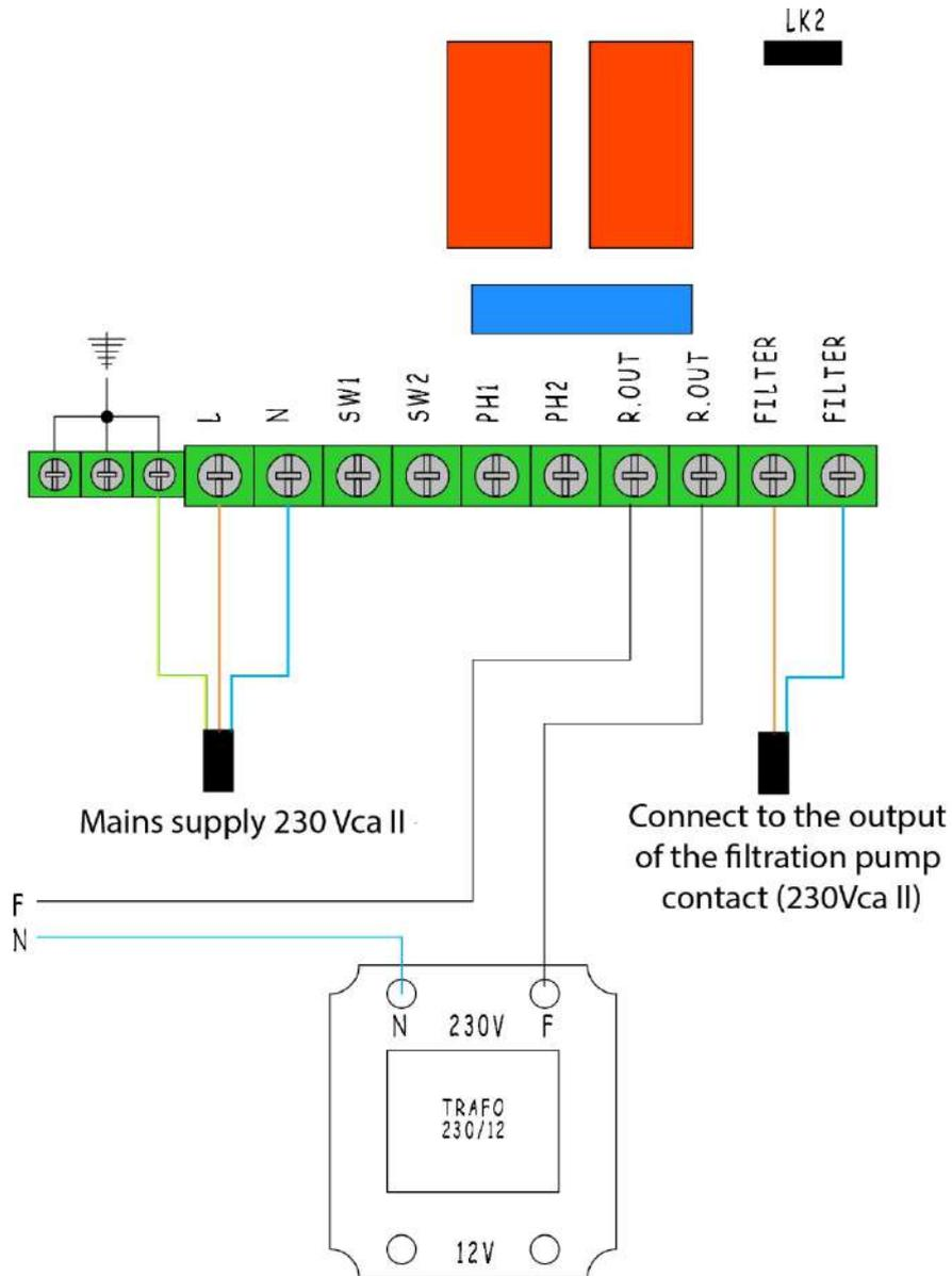
Attention: Never exceed 12A when using the auxiliary relay. For higher currents, supplement the circuit with a contactor.
