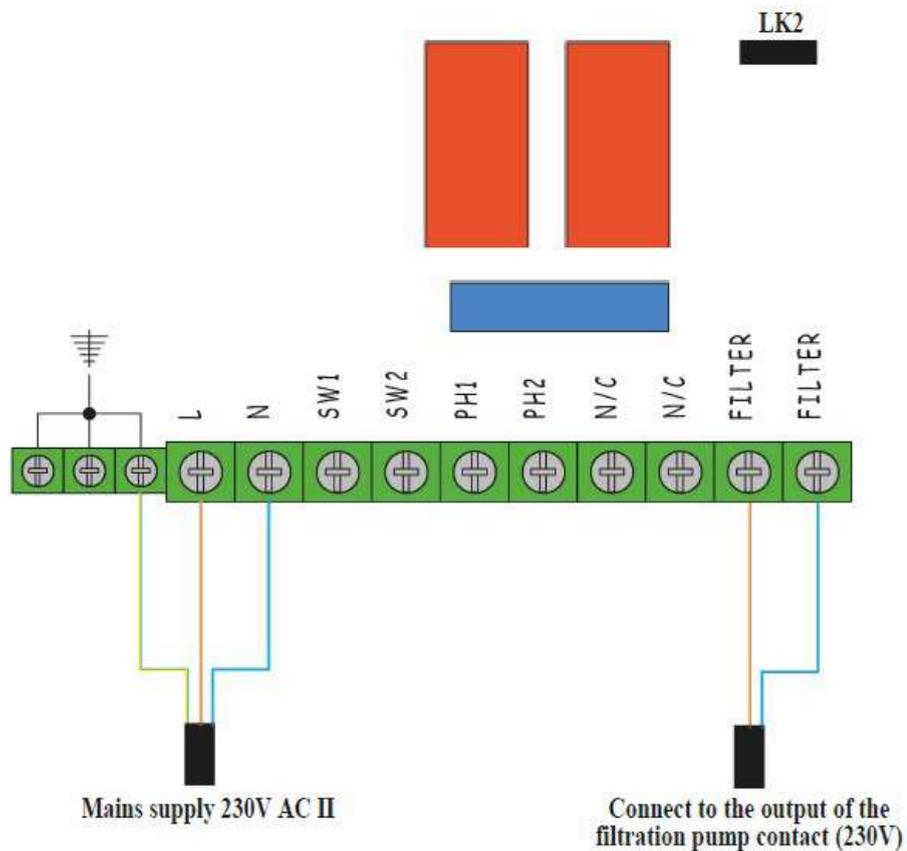
3.3.3.2- Programming the spotlights of the pool through the auxiliary relay
