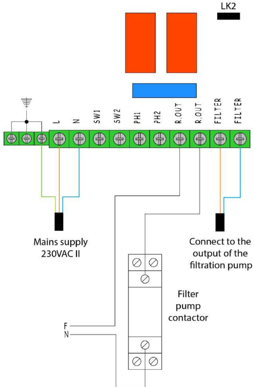
Please remember that the equipment should be configured in "start-stop" mode, as detailed on section 3.3.2.1.
