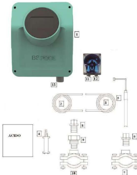
Once the equipment (1) is installed, the following connections should be done.
