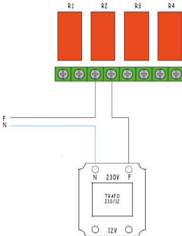
Attention: Never exceed 5A when using the programmable relay. For higher currents, supplement the circuit with a contactor.
