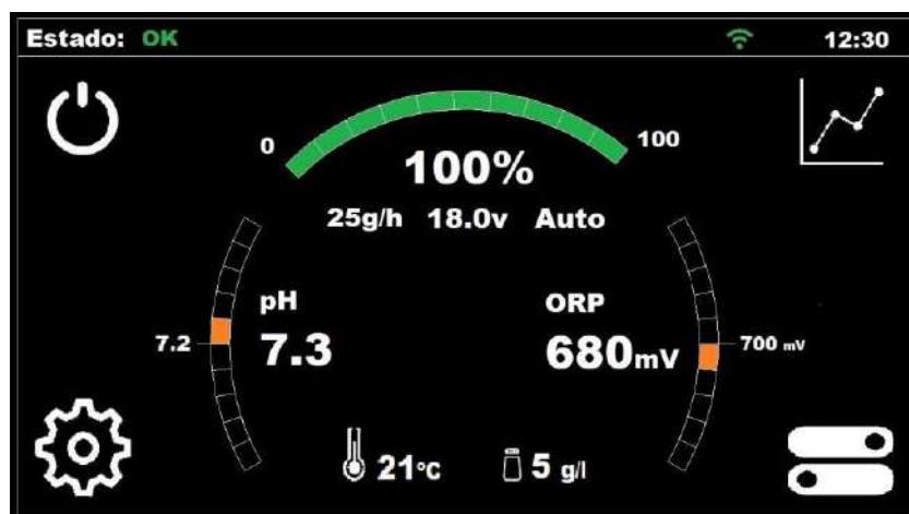
On the uppermost part of the screen, you can see the display status bar. The left side of this bar shows the actual status of the chlorinator. On the right you can see the current time of day once it is correctly configured. You can also see the connectivity status of the equipment EYPOOLS (EYP-004).
