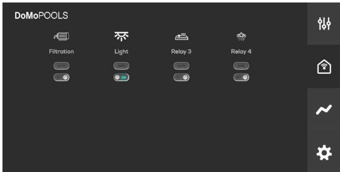
Press ON/OFF for manual control. If AUTO mode is required, click on the relay icon a set a program cycle.
