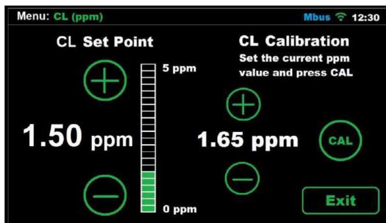
In this case, the ppm value can be adjusted within a 0-10ppm range.
