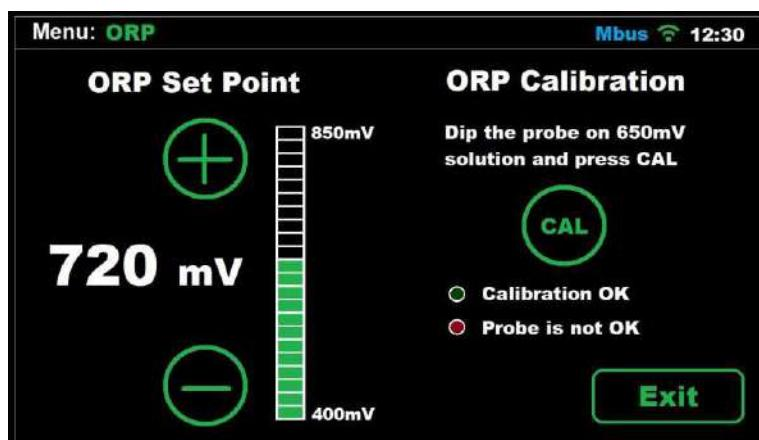
To Access the **ORP Menu**, touch the ORP measurement value on the **Main screen**.
