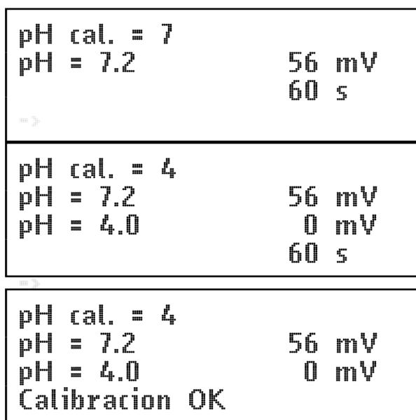
At the end of the 60 seconds, the message "Calibration OK" will appear. Press "OK". If an error message appears, it may be due to a dirty (see maintenance) or defective probe, contaminated standard solutions or a bad connection.
