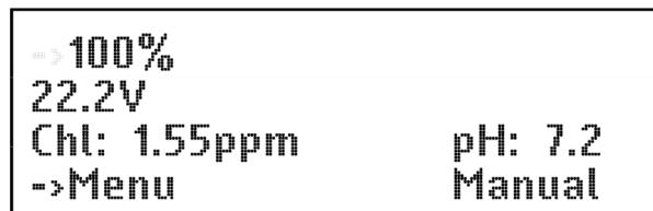
The upper line shows the production % of each installed power supply.
