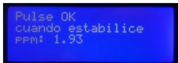
Adjust the real value obtained by means of DPD-1 test.
