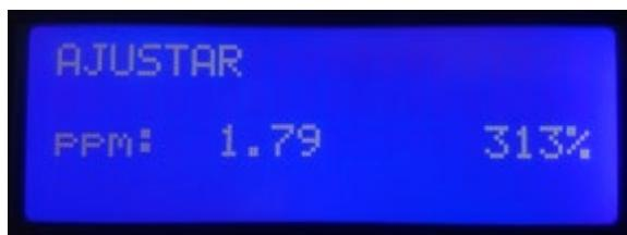
Return to the main screen. The current CL value will match with the value obtained from DPD-1 test.
